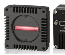
Line scan cameras are a type of camera that captures images one line at a time, unlike regular cameras that capture entire frames at once. They work by using a linear sensor of 1 or 2 pixels high that scans across the field of view. The motion of the sensor or the object being captured creates the second dimension of the image, building up the image one line at the time.
