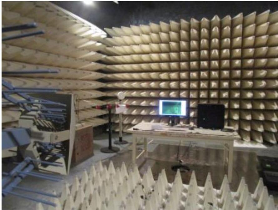
**Photograph 4: Set-up for immunity test of fast transient/burst**
