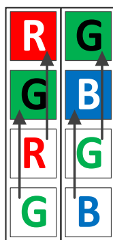
Figure 8-34 Vertical color Binning by 2
