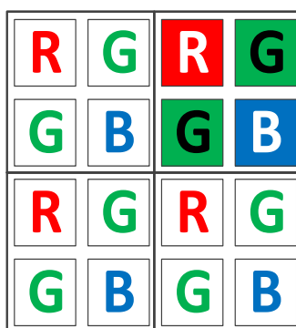
Figure 8-35 Horizontal and vertical color Binning by 2x2
